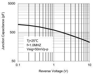
Fig.5 – Typical Junction Capacitance
