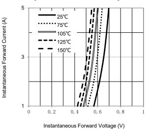
Fig.3 – Typical Forward Voltage Characteristics
