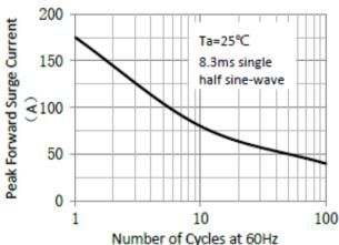
Figure 2.Maximum Non-Repetitive Peak Forward Surge Current
