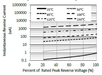
Figure 3. Typical Reverse Characteristics
