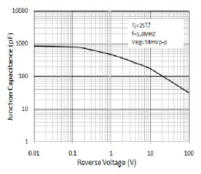
Figure 5. Typical Junction Capacitance
