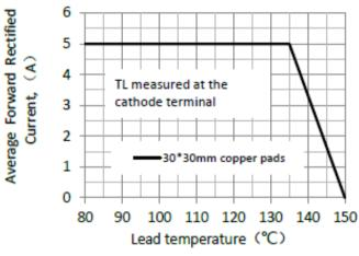
Figure 1. Forward Current Derating Curve
