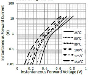
Figure 4. Typical Instantaneous Forward Characteristics
