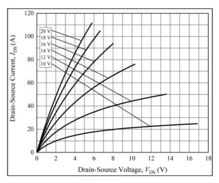
Figure 2. Typical Output Characteristics at TJ = 25 ℃
