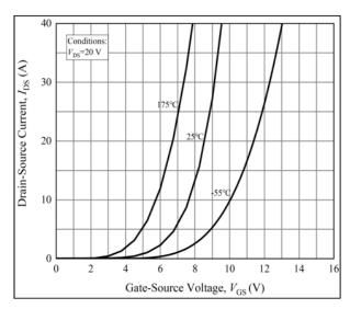
Figure 4. Typical Transfer Characteristics for Various Temperature
