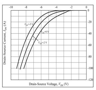
Figure 8. Typical Body Diode Characteristics at TJ = -55  $^{\circ}$ C
