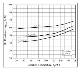
Figure 7. On-Resistance vs. Temperature for Gate
