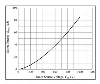
Figure 16. Typical Output Capacitor Stored Energy
