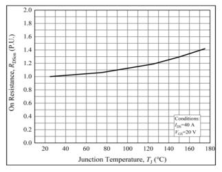
Figure 5. Normalized On-Resistance vs. Temperature
