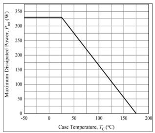
Figure 19. Power Dissipation Derating Curve
