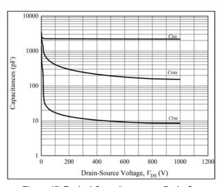
Figure 17. Typical Capacitances vs. Drain-Source Voltage
