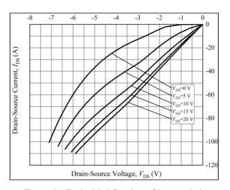
Figure 15. Typical 3rd Quadrant Characteristics at TJ = 175  $^{\circ}$ C
