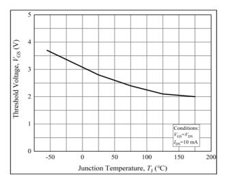
Figure 11. Typical Threshold Voltage vs. Temperature
