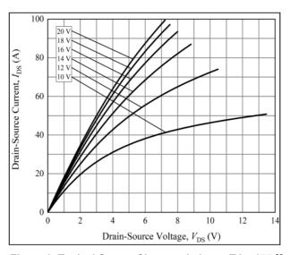
Figure 3. Typical Output Characteristics at TJ = 175  $^{\circ}$ C
