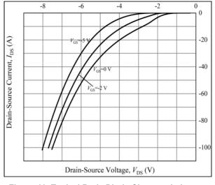
Figure 10. Typical Body Diode Characteristics at TJ = 175  $^{\circ}$ C
