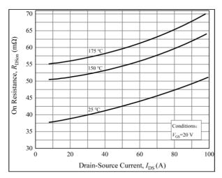
Figure 6. On-Resistance vs. Drain Current for Various Temperatures
