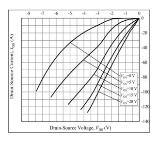
Figure 14. Typical 3rd Quadrant Characteristics at TJ = 25  $^{\circ}$ C
