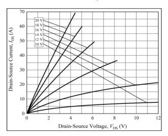
Figure 1. Typical Output Characteristics at TJ = -55 ℃
