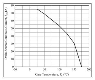
Figure 18. Continuous los Current Derating Curve
