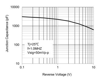
Fig.5 – Typical Junction Capacitance
