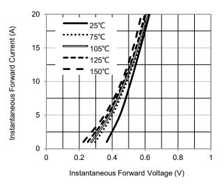
Fig.3 – Typical Forward Voltage Characteristics
