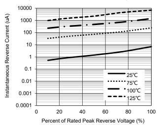
Fig.4 - Typical Reverse Current Characteristics
