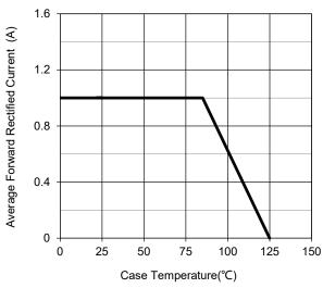
Fig.1 - Forward Current Derating Curve
