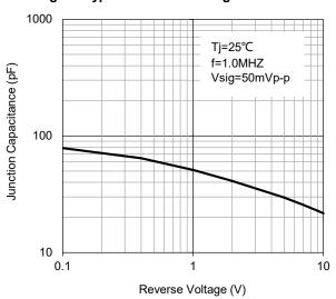
Fig.5 - Typical Junction Capacitance
