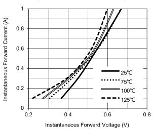
Fig.3 - Typical Forward Voltage Characteristics
